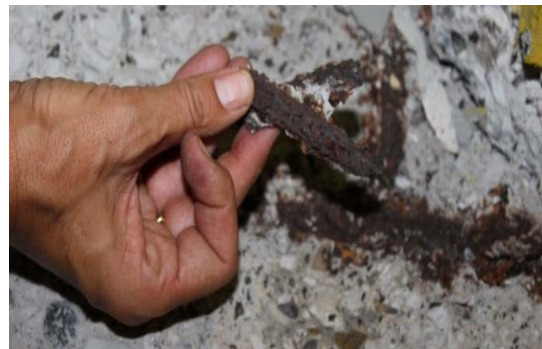
Figure 1 – Left: Successful selfhealing of crack at concrete. Right: Heavy reinforcement corrosion at bars at unhealed cracks.
